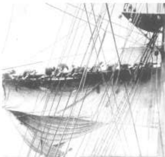
Working at the mainsail in calm. The set of sails was replaced by a heavier one before reaching Cape Horn; later they were changed again.
