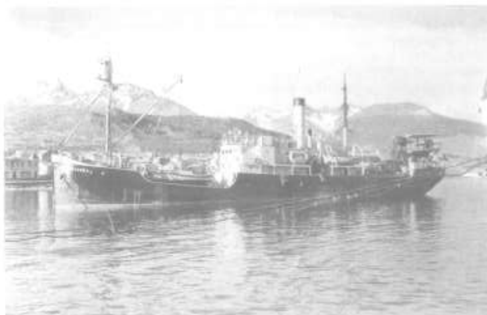
Transport 'Patagonia' with a hydroplane at stern and a bird's nest top of the foremast to descry ice during the Antarctic Campaign.
