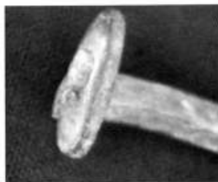
Figura 17: Detalle de la punta remachada. Figure 17: Clinched tip detail.
